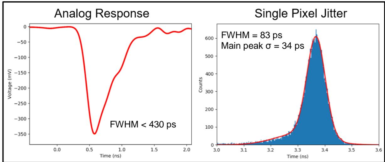
*Figure 1: (Left) Average of 50 pulses measured on a 5 GHz oscilloscope, using an LPG-405 pulsed laser. (Right) Histogram of 5,000 single-photon pulse arrival times measured with an attenuated LPG-405.*
