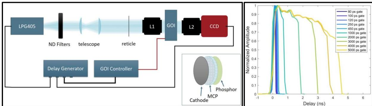
**Figure 2: (Left) Schematic for a gating characterization measurement of a gated optical imager (GOI). (Right) Data acquired with an LPG-405 being sent to Sydor's Picosecond Gated Optical Imager (ps-GOI).**
