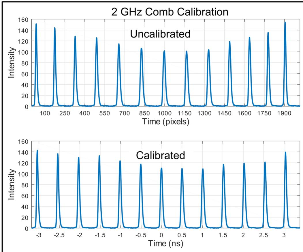
*Figure 5: 2 GHz comb shown in an uncalibrated (top) and calibrated (bottom) lineout from a system data test at the factory.*
