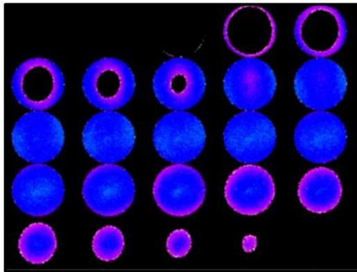
Figure 3: Effect of irising as seen in an MCP118 with a 4 ns gate window. Each step represents 200 ps delay of the laser.
