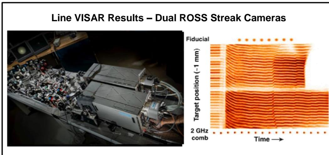
Figure 4: (Left) Streak camera benchtop setup for VISAR. (Right) Streaked image showing interferometer fringes, a facility fiducial (top), and a built-in comb reference (bottom).
