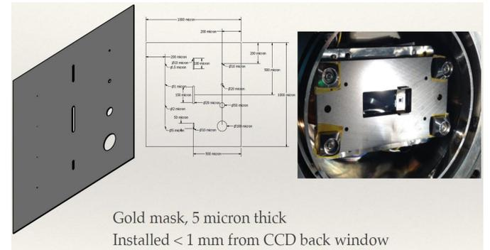
Figure 4 Gold mask with different features to measure the position resolution of the Spectro CCD with low flux soft x-rays.
