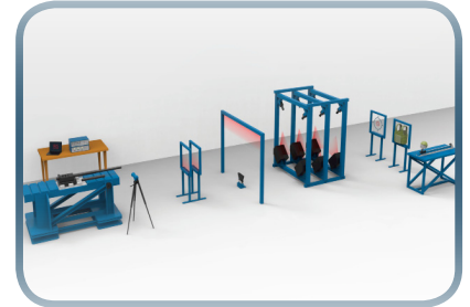
Sample range design: test gun and stand, IR muzzle flash sensor, velocity measurement equipment, Y.A.W. measurement system, targets, and readout electronics.
