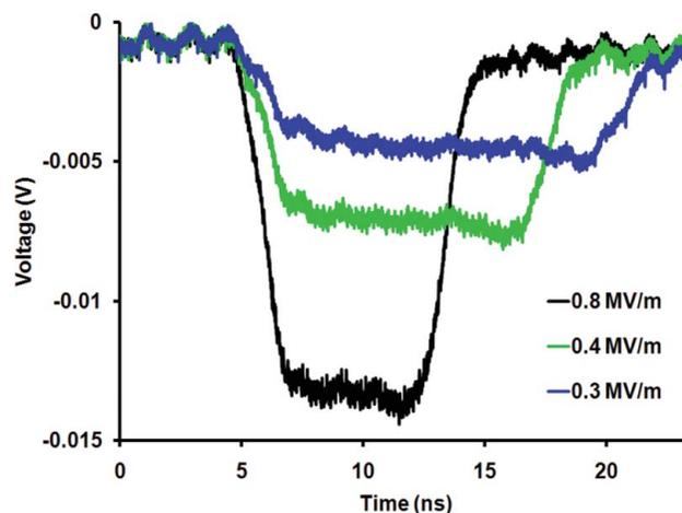
**Figure 9** Pulse width as a function of field in the diamond. This measurement uses broadband soft X-rays (0.2–1 keV). Increased field decreases the carrier transit time. The voltage is measured into  $50 \Omega$  using a  $\times 10$  amplifier.
