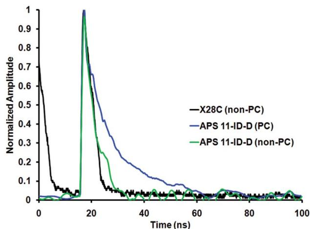
**Figure 8** Normalized timing measurements performed at the APS. Non-PC (green) and PC (blue) diamond exposed to monochromatic (12 keV) X-rays at 11-ID-D ( $0.7 \text{ MV m}^{-1}$  field). The non-PC timing measurement ( $2 \text{ MV m}^{-1}$  field) for the high-flux X-ray white beam at X28C (black) is included for comparison.
