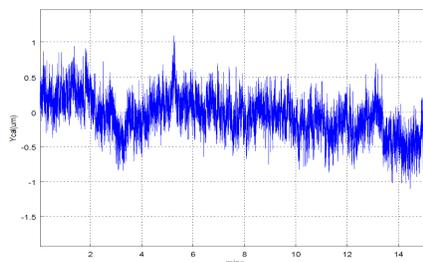
Fig. 5 Vertical x-ray beam motion observed over a 15 minute period
