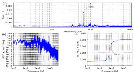
Fig.9 Measured vertical beam motion: (a) Fast Fourier Transform (b) Power spectrum (c) Frequency contribution to vertical beam motion.
