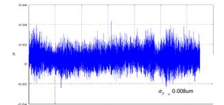
Fig.8 10kHz data of beam vertical motion
