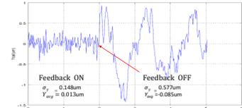
Fig. 7 Vertical beam stability with the SIEPA3P feedback control enabled and then disabled.
