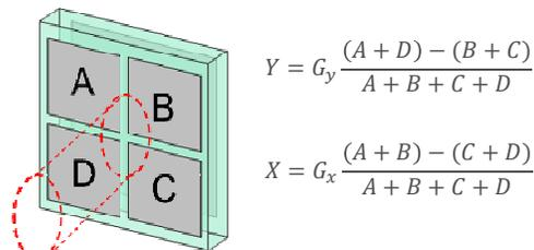
Fig. 2 Quadrant Diamond BPM (Left). The charge collected by each quadrant is utilized to calculate the x-ray beam position via a difference over sum algorithm (Right)
