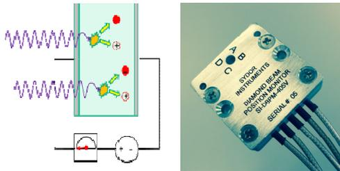
Fig. 1 Electron-hole pair production in CVD diamond (Left). Sydor DBPM (Right).
