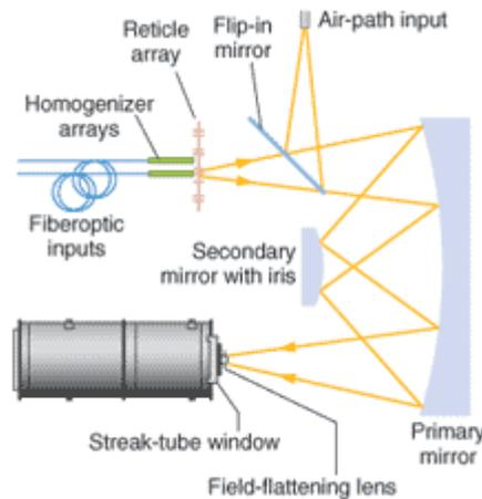
*Input optics for the ROSS camera are based on an Offner triplet system. An air path for signals from external sources can be selected with a flip-in mirror, or the homogenizer arrays for fiberoptic signals and internal calibration sources can be used.*
