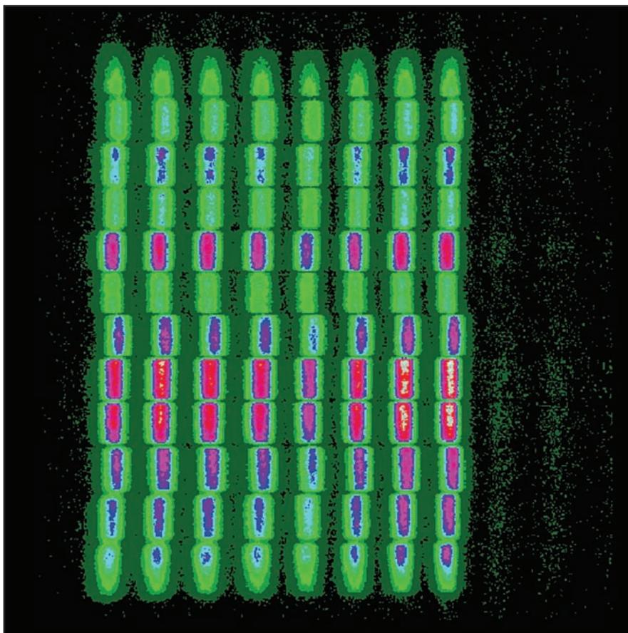
**Figure 2.** This streak calibration image was taken using a slow ramp technique. Spatial information is taken at several points in the image and then processed to characterize the geometrical distortion and flat fielding profile.
