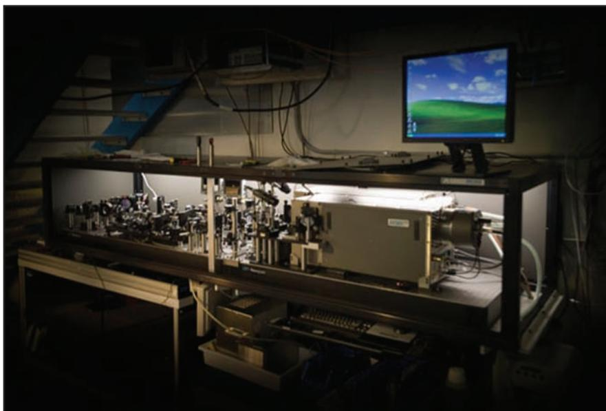
**Figure 3.** An active shock breakout diagnostic is shown on the Omega laser at the University of Rochester Laboratory for Laser Energetics. Sydor built the system, which consists of a pair of streak cameras and velocity interferometers to image laser-driven shock waves for inertial confinement fusion research.
