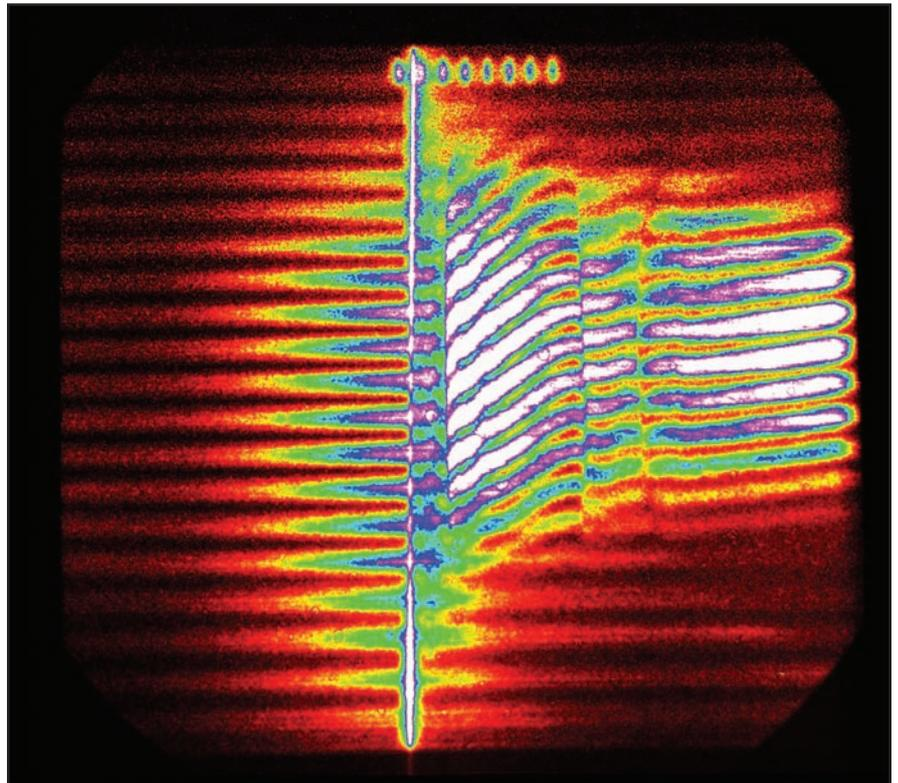
**Figure 1.** In this streak image taken with a velocity interferometer and self-calibrating streak camera, fringe transitions show the breakout of a shock wave on ultrafast timescales. Note the timing reference signal at the top of the image.
